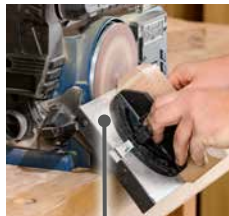
Supporting table can be tilted
