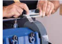
Universal jig designed for many straight standard tools
